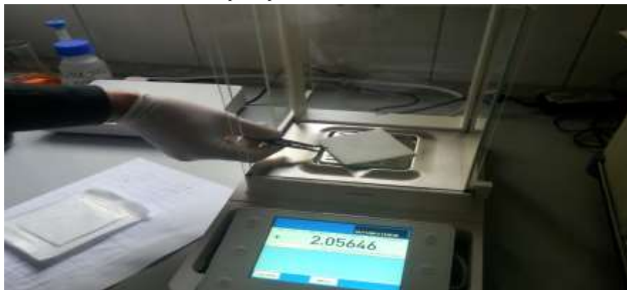
Figure 1: Instrument CUBIS Sartorius MSA 225 S in six decimals
