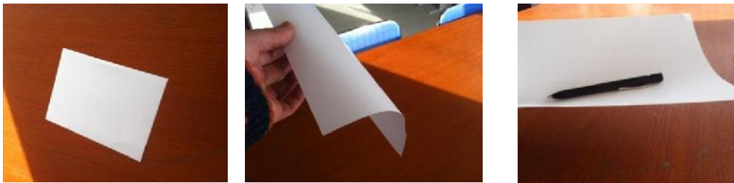
Fig. 1. 1 Left: A4 sheet of paper in plane ( \rho = 0 ); in the middle: A4 sheet given a certain curvature \rho = \rho_0 ; right: the generated cylindrical surface and the shear increase of the bearing capacity ( \rho = \rho_0 ).
