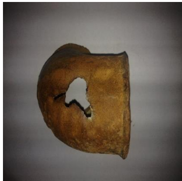
Fig.5a Pipeline and flow apacity in different holes, 5b. Pipe age and high level corrosion in metal pipes. 5c Graph Moody Diagram
