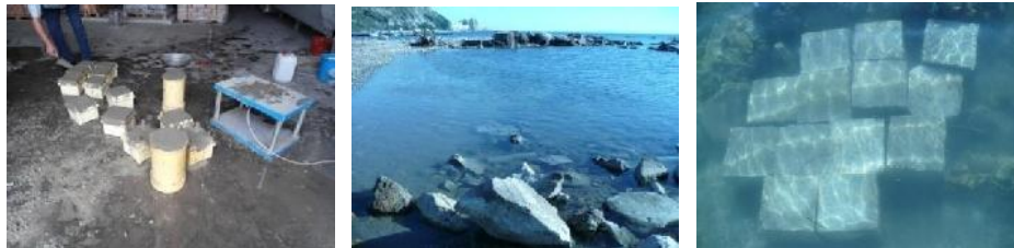
Fig. 3. Concrete specimens produced in Euro Aditiv Laboratory and curing in the sea shore of Durres city, Albania
