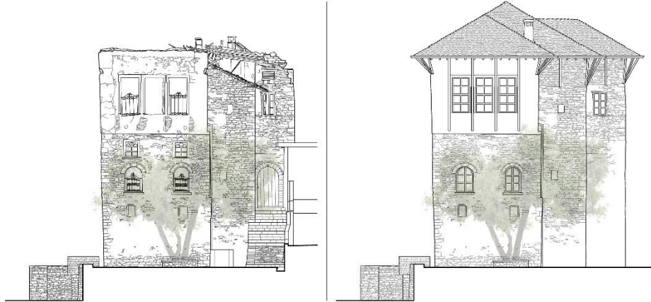
Fig. 2. Main façade of the Kokalari House now and after the major repair
