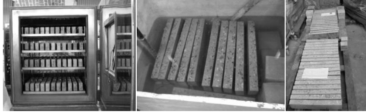
Figure 6 (left) Climatic chamber; (middle) Water immersion; (right) air exposure
