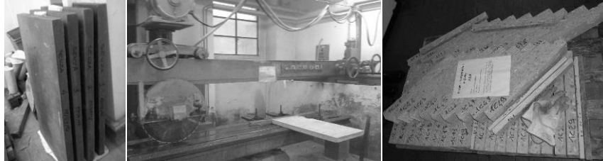
Figure 4. (left) Slabs stored on a chamber room; (middle) cutting machine; (right) specimens like “beam” after cutting
