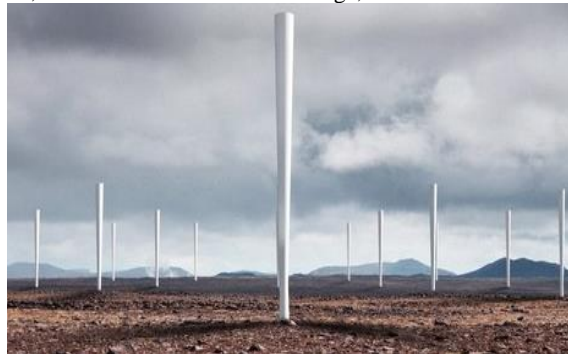
Figure 4: The Vortex of wind turbine being developed without any blades.
