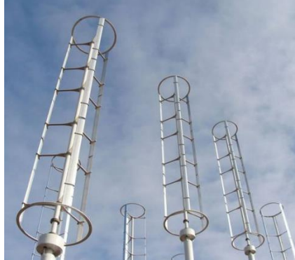
Figure 5: Wind spire vertical Axis Turbines
