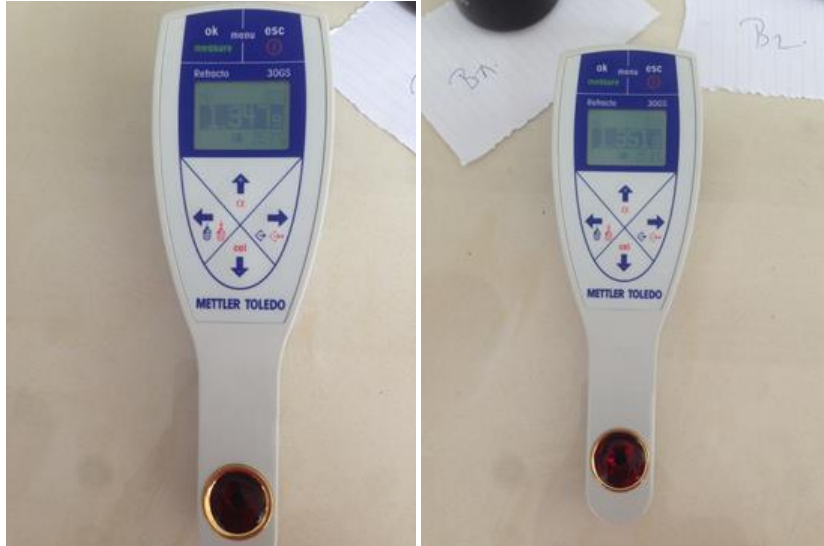
Fig. 2. Determination of refractive index and dry matter
