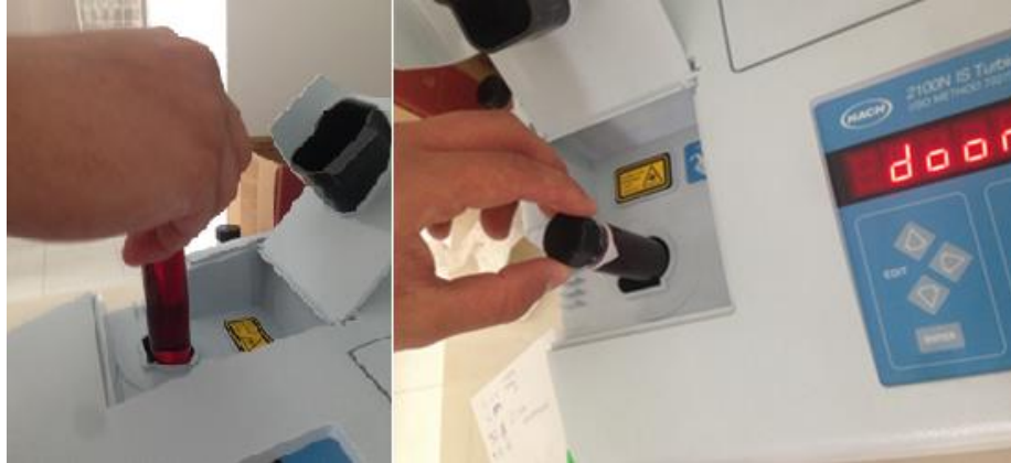
Fig. 5. Determination of turbidity (NTU)
