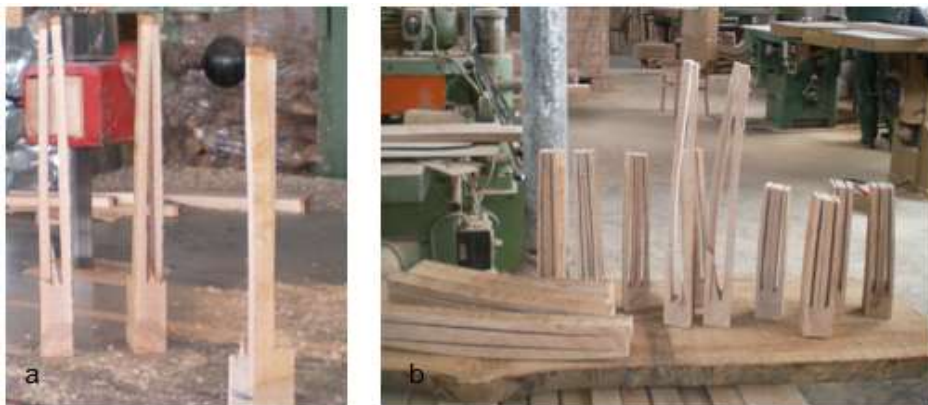
Fig 7. Samples for prongs probes with different thickness
