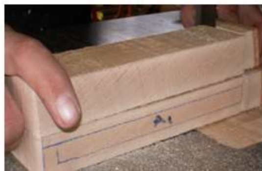
Fig 4. Method of cutting section for measuring shell and core moisture content. (ML88 5586). a. for thickness 25-37 and 38 to 49 and b. for thickness 50 to 70
