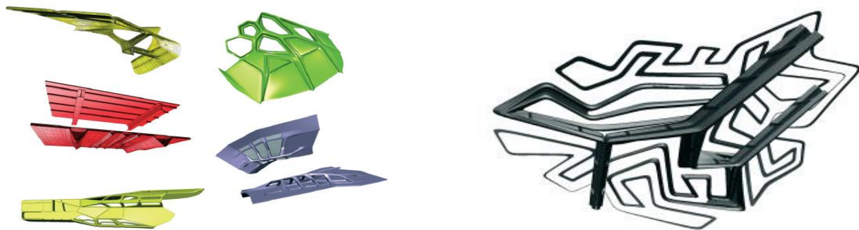
Figure 5.4.2: (left) EMERGENT, the Menagerie, 2006 - Integration of "air flow" ducts within a hybridized component with the structure of the building. (right) EMERGENT, Lizard Panel Facade, 2009 – Façade prototype combining a greywater capture system with an algae photo-bioreactor system in a way that produces structural as well as ornamental effects. (Credits: © Architectural Design (2010) 'Exuberance' Vol 80/2, Wiley Academy, p. 80 – 83)
