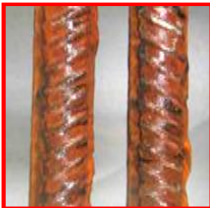
Figure 7. Appearance of carbon steel after three weeks of exposure.
