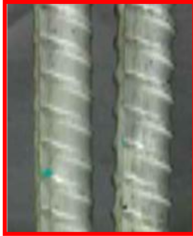
Figure 5. Appearance of stainless steel 316LN after three weeks of exposure.
