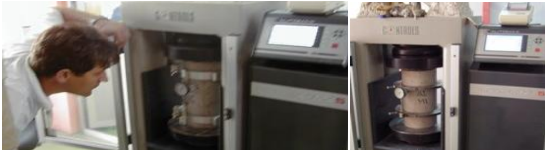
Fig. 4 Testing of Modulus of elasticity
