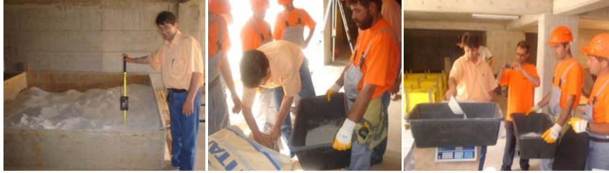
Fig. 2 Measurement of the integral components of concrete
