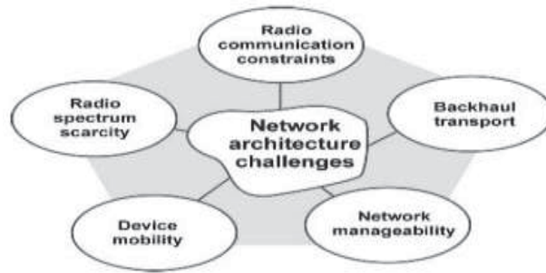
Fig. 4. Challenges of a mobile network design [Source: Wiley 2005, “UMTS architecture Mobility and Services”]
