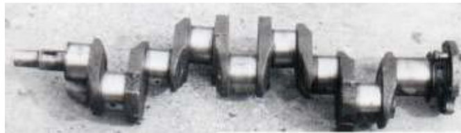
Fig. 1. The crankshaft of tractor 75 D
