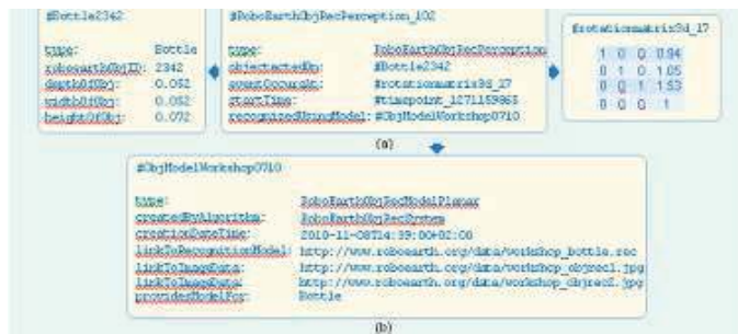
Fig. 3. The object description, recognition model, and one particular perception instance of the bottle used in the second demonstrator [8]
