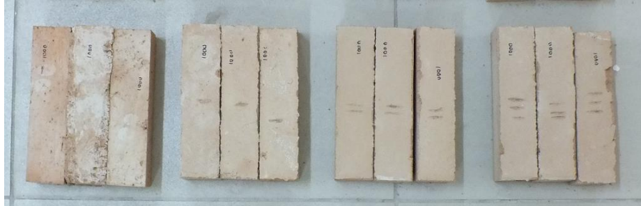
Fig. 3. Specimens with coal powder additive (from left to right M0, M10, M20 and M30)
