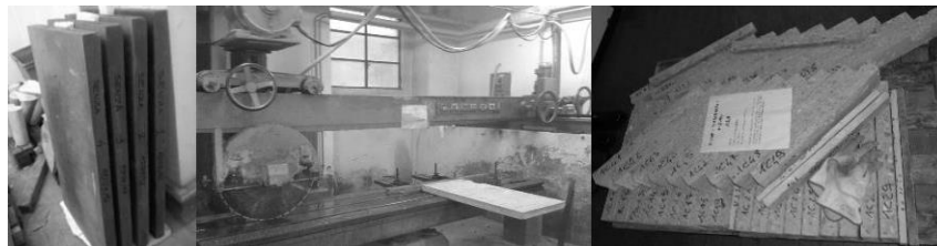
Figure 4. (left) Slabs stored on a chamber room; (middle) cutting machine; (right) specimens like “beam” after cutting
