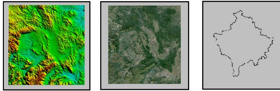
a) Derived USGS DEM file b) Image raster file c) MapInfo vector file Fig. 16. a), b) and c) Input data for workflow in FME
