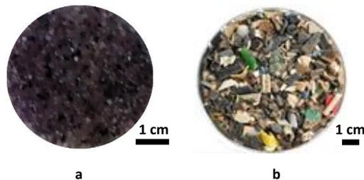
**Fig. 1.** Polished section of a milled product (-1100 +600)  $\mu\text{m}$  as resulting from the mechanical processing of a porphyry copper ore (a) and +10 mm bulk WEEE products fed to Magnetic Density Separation (MDS) (b).
