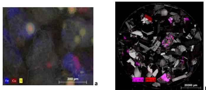
**Fig. 3.** XRF elemental maps of a polished section ROI (Region of Interest) identifying Cu and S of chalcopyrite grains (a) and metallic elements mainly occurring in Printed Circuit Boards (PCBs) (b) of +10 mm bulk WEEE products fed to MDS.  $\mu$ -XRF analyses were performed using a benchtop XRF spectrometer (M4 Tornado, Bruker®). Elemental maps are the results of a XRF peak deconvolution of the sum spectra collected pixel by pixel.
