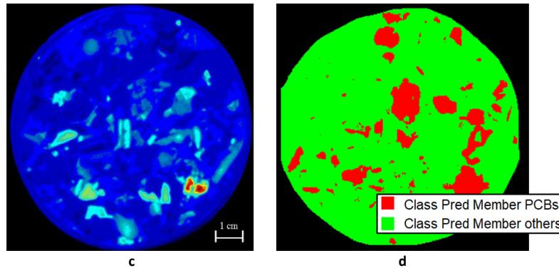
**Fig. 5.** Mean reflectance hyperspectral image (1000 – 2500) nm of the +10 mm bulk WEEE products fed to MDS (a) and the related PLS-DA prediction map identifying the PCBs (b). Analyses have been carried out utilizing a SISUChem XLTM Chemical Imaging Workstation (Specim, Finland), equipped with an ImSpector™ N25E imaging spectrograph working in the 1000-2500 nm wavelength range.
