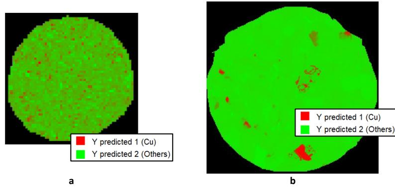
**Fig. 4.** a: PLS-DA copper prediction maps as resulting from the XRF mapping of -1100 + 600  $\mu\text{m}$  polished sample of particles containing and gangue minerals (a) and of the +10 mm bulk WEEE products fed to MDS (b).
