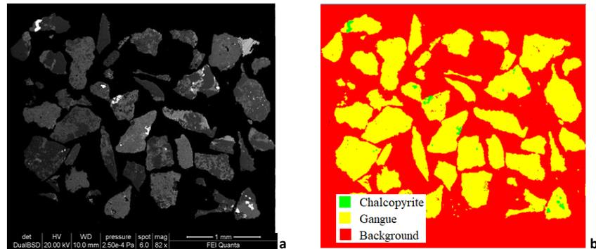
**Fig. 2.** SEM–BSE image acquired at 82 x for -1100 + 600  $\mu\text{m}$  polished sample of particles containing chalcopyrite (a) and RGB image, segmented by thresholding, processed in Image-Pro® Plus (a). SEM analyses have been carried out using a Hitachi S2500 SEM equipped with a EDS-KeveX 8000 microanalysis unit with a Si(Li) detector.
