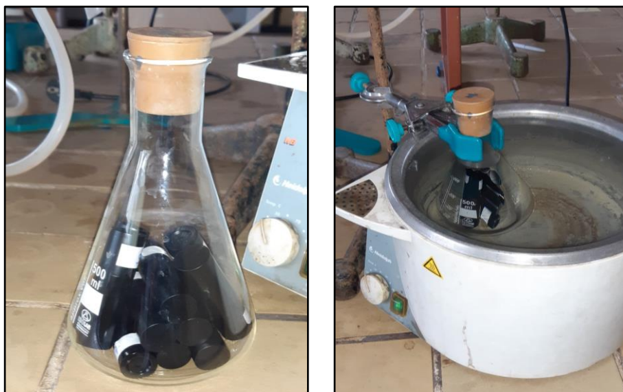
Fig 3. Measurement of temperature stability \approx 45\text{ }^{\circ}\text{C}
