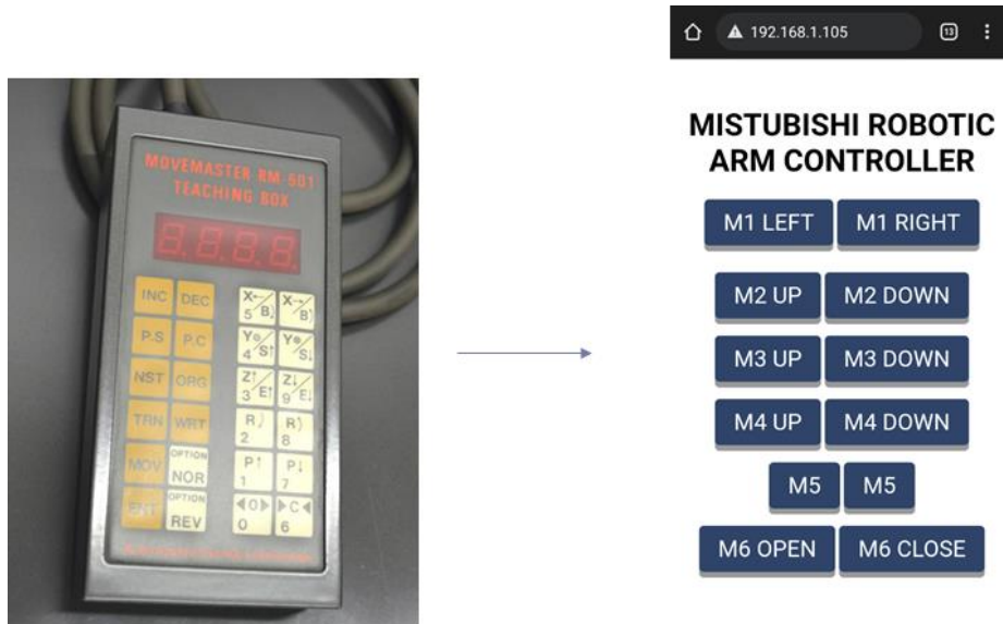
Figure 3. Old control interface (on the left) vs new web-based control interface (on the right)
