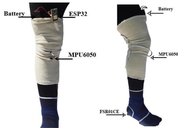
Figure 1: Implementation of sensors and Esp32 in the knees.
