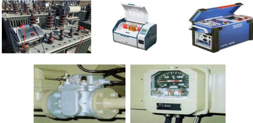
Fig. 4. (a) Insulation resistance test of 10/0.4 [kV] transformer; (b) Equipment for testing the dielectric strength of oil; (c) OMICRON CPC 100; (d) Buchholz relay and (e) Thermometer
