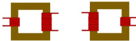
Fig. 1. Winding of step-up and step-down transformers
