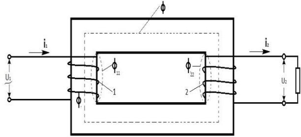
Fig. 2. The operation principle of the transformer
