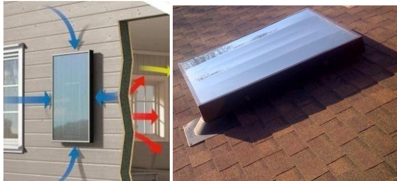
Fig 2. The structure of air solar collector [8].
