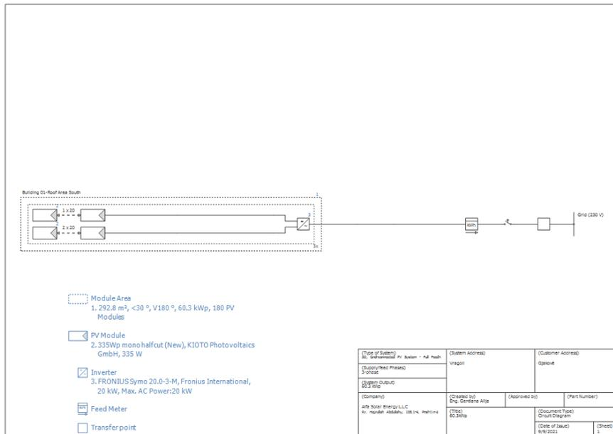
Fig. 4.3. One-time diagram of the PV system
