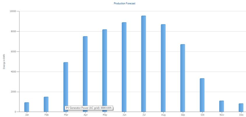
Fig. 4.4. Predicting energy production during design with PVSOL\*Premium
