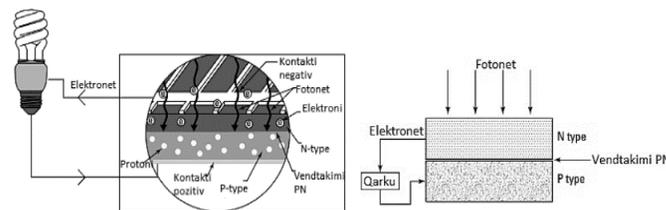
Fig. 3.1. Photovoltaic current generation
