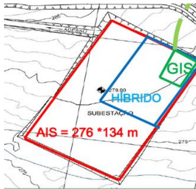
Fig.7. Space covered by a GIS System vs AIS System
