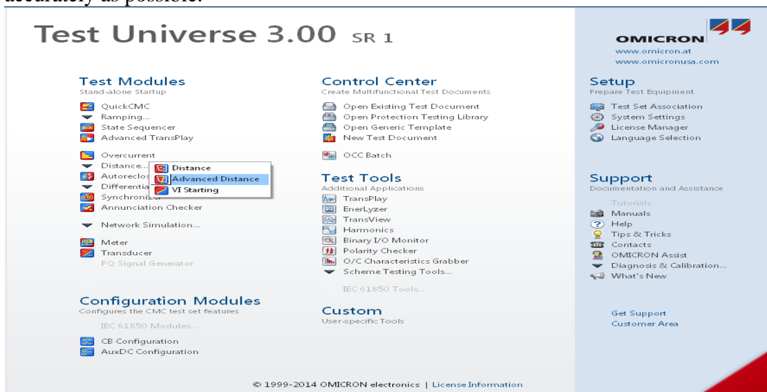
Figure 2 The first page of testing a remote protection
