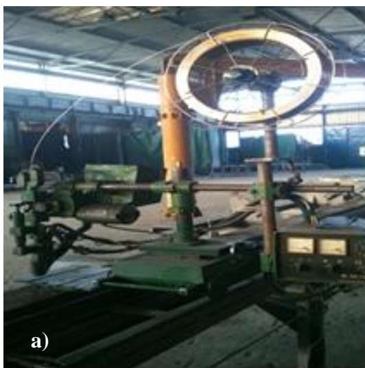
Fig 1. a) submerged arc welding machine b) wire and OK Flux 1071 [7].
