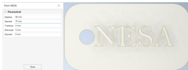
Fig. 3. The result we will have when the "Gjeresia" values are greater than 70 and less than or equal to 75 (Material: Aluminum 6061, Color: Silver)
