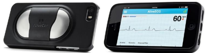
Figure 8. Sensor for EKG monitoring in the form of a phone case.
