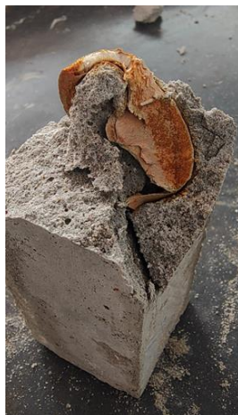
Fig. 5. Matrix/Endocarp interface Source: From the authors (2023)
