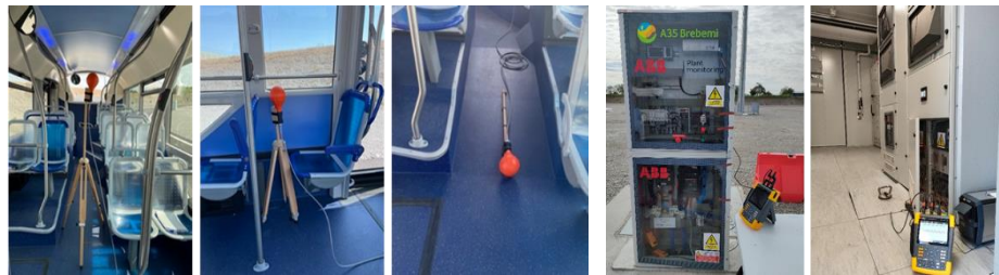
Fig. 2. Measurement of magnetic field on board of the vehicle (left) and measurement system of electric quantities in the correspondence of MU and in AC/DC substation (right)
