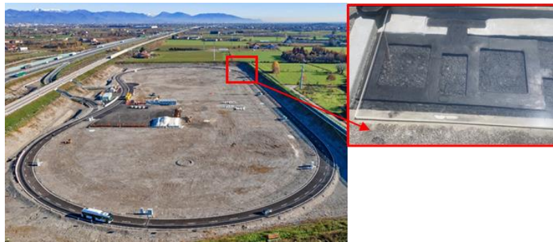
Fig. 1. Trial field photography with vehicles on the road: Iveco Intercity Bus and Fiat 500 utility car; Zoom Fig. 1. Detail of a portion of the ring track pavement where the electromagnetic coil used for wireless charging is visible.
