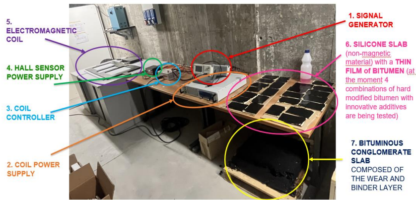
Fig. 3. Instrumentation and scheme of work for the reproduction of the DWPT system in the laboratory
