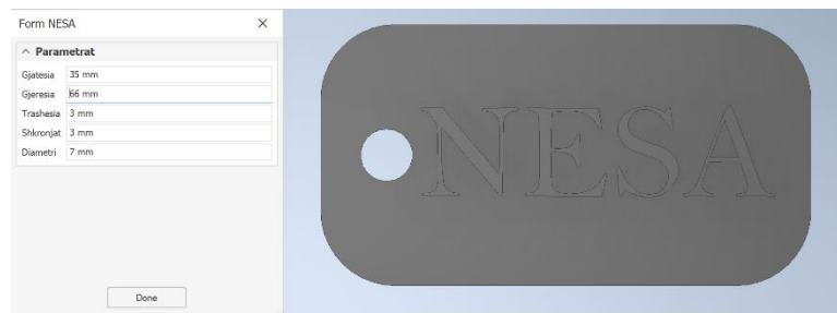
Fig. 2. The result we will have when the "Gjeresia" values are greater than 65 and less than or equal to 70 (Material: PLA Plastic, Color: Dark Grey)
