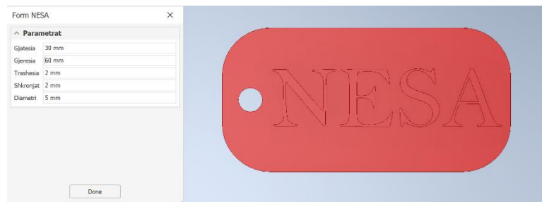
Fig. 1. The result we will have when the "Gjeresia" values are greater than or equal to 60 and less than or equal to 65 (Material: ABS Plastic, Color: Red)
