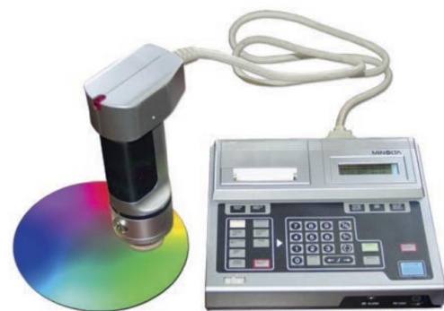
Figure 2 - Konica Minolta colorimeter. It measures the color by means of three sensors with the tristimulus method, therefore it is more limited than the spectrophotometer.
